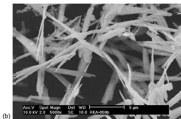
Fig. 1. SEM micrograph of [Al]-SSZ-31 zeolite. (a) DGC (DG2, \text{SiO}_2/\text{Al}_2\text{O}_3 = 176 ); (b) HTS (HT2, \text{SiO}_2/\text{Al}_2\text{O}_3 = 235 ).
